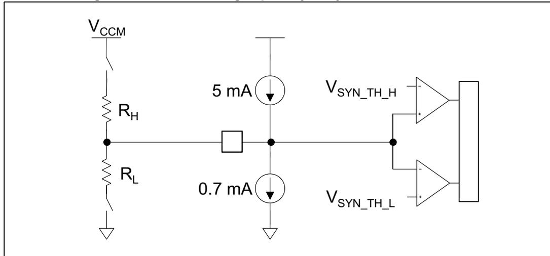
As anticipated above, in SLAVE mode the internal oscillator operates at 250 kHz typ. but the slope compensation is dimensioned accordingly with FSW resistors so, even if the A6986 supports synchronization over the 275 kHz - 1.4 MHz frequency range, it is important to limit the switching operation around a working point close to the selected frequency (FSW resistor).
