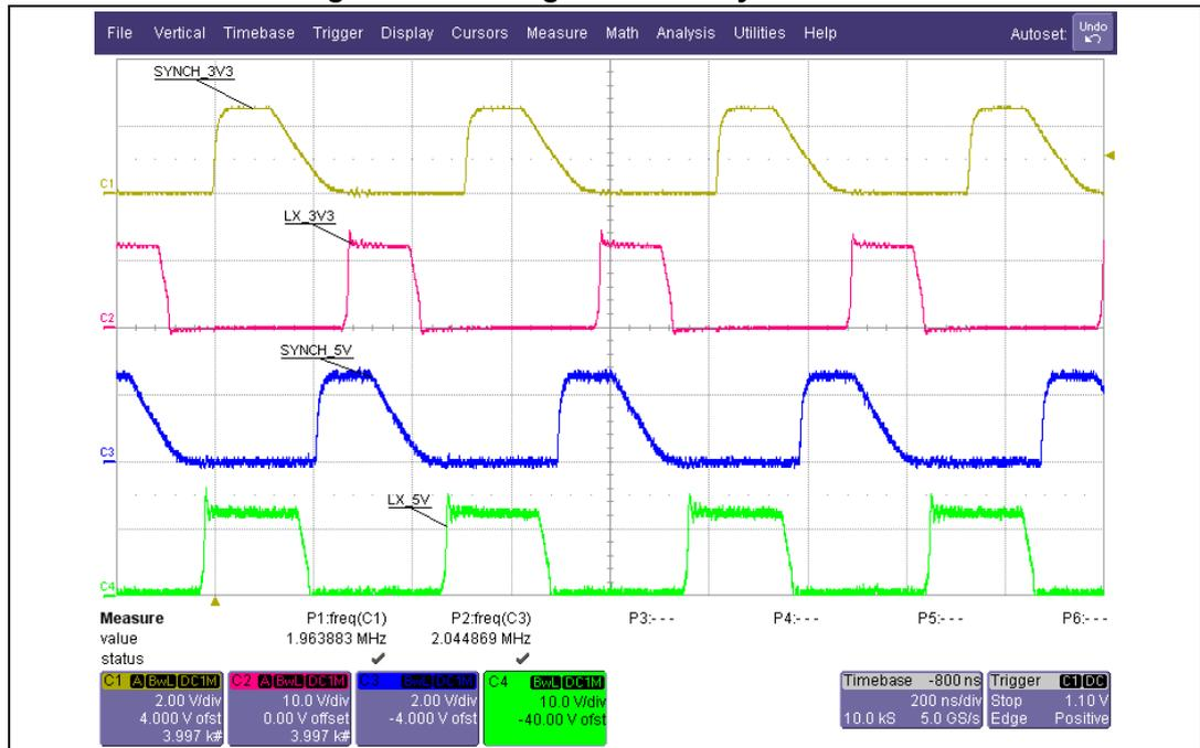
Figure 33 shows the same regulators working synchronized. The MASTER regulator (LX2 trace) delivers the synchronization signal (SYNCH1, SYNCH2 pins are connected together) to the SLAVE device (LX1). The SLAVE regulator works in phase with the synchronization signal which is out of phase with the MASTER switching operation.
