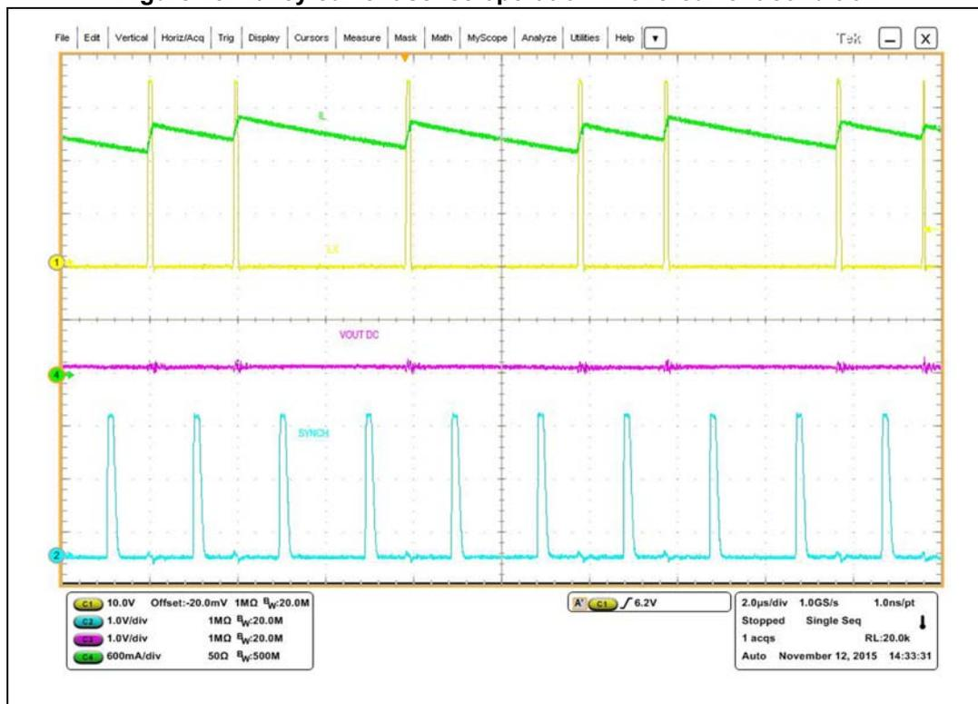
Figure 18 shows the switching frequency reduction during the valley current sense operation in case of extremely low duty cycle ( $V_{IN} = 38\text{ V}$ ,  $f_{SW} = 500\text{ kHz}$  short-circuit condition).
