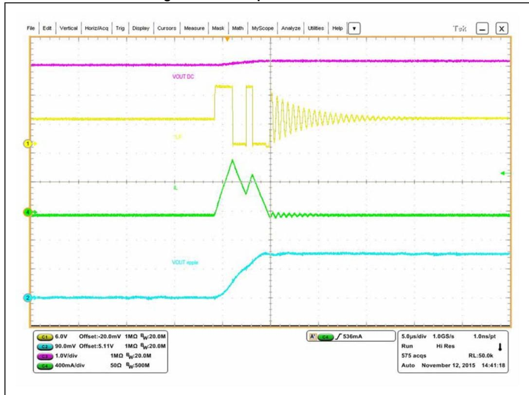
Given the energy stored in the inductor during a burst, the voltage ripple depends on the capacitor value:
