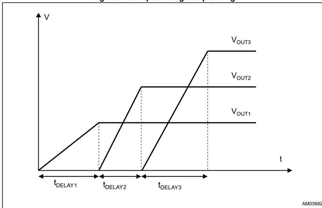
High flexibility is achieved thanks to the programmable RST thresholds (see [Table 7: LNM / LCM selection on page 12](#)) and programmable delay time. To minimize the component count the DELAY pin capacitor can be also omitted so the pin works as a normal power good.
