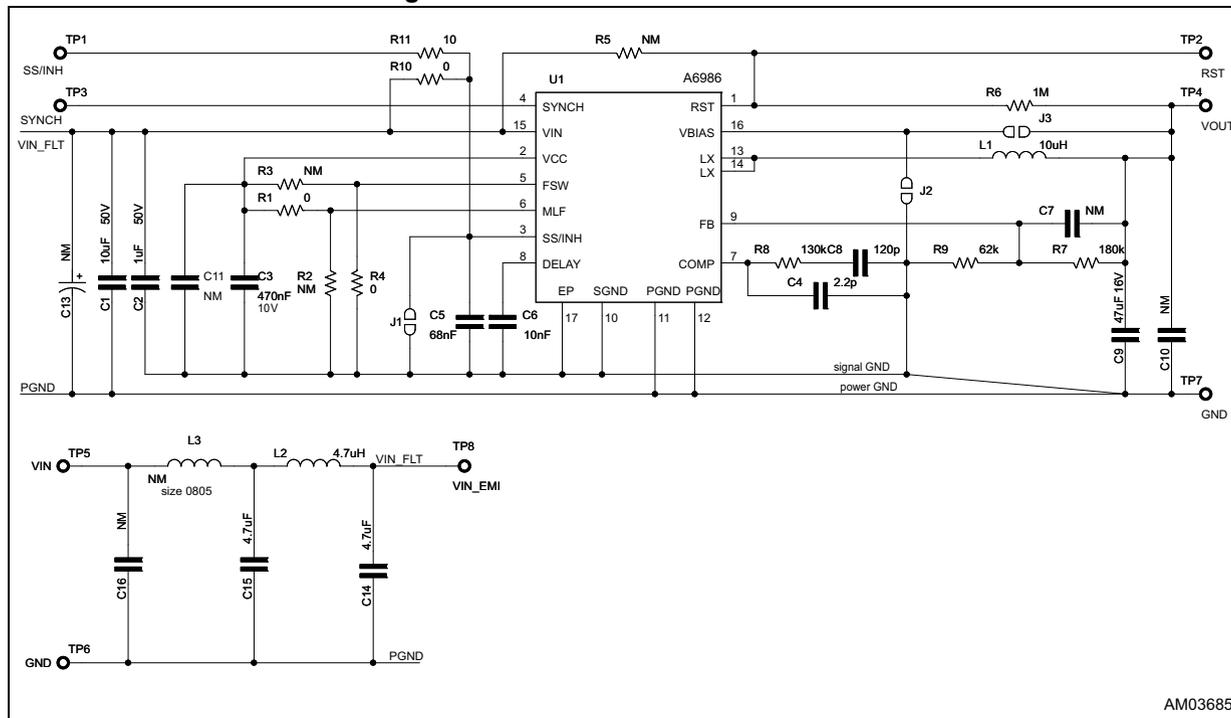
The additional input filter (C16, L3, C15, L2, C14) limits the conducted emission on the power supply.
