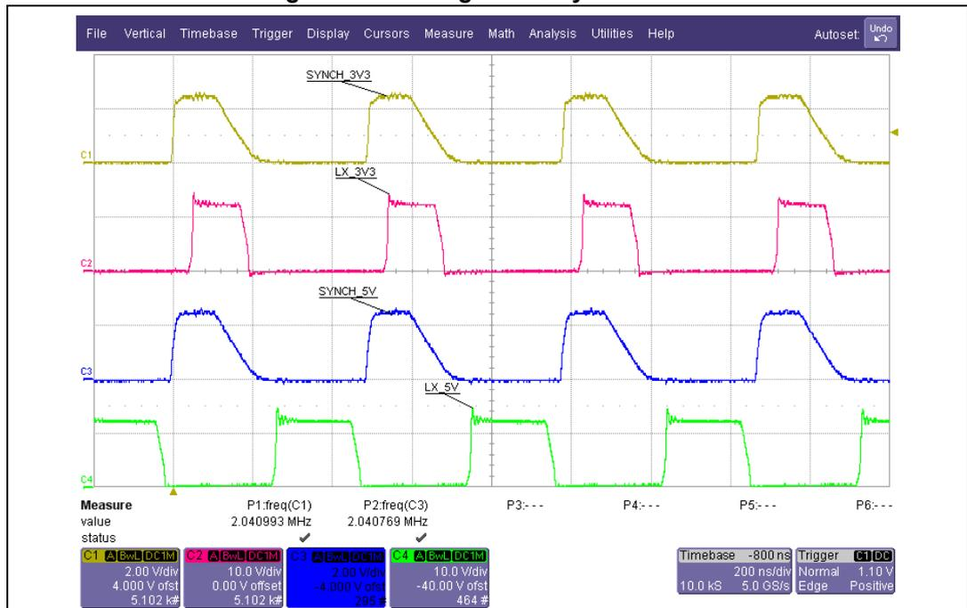
Multiple A6986 can be synchronized to an external frequency signal fed to the SYNCH pin. In this case the regulator set is phased to the reference and all the devices will work with 0° phase shift.
