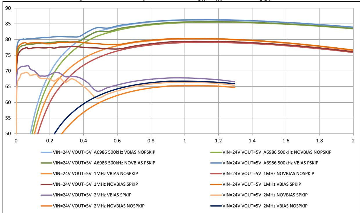
Figure 50. Efficiency curves over  $f_{sw}$ :  $V_{IN} = 24\text{ V} - V_{OUT} = 5\text{ V}$  (log scale)
