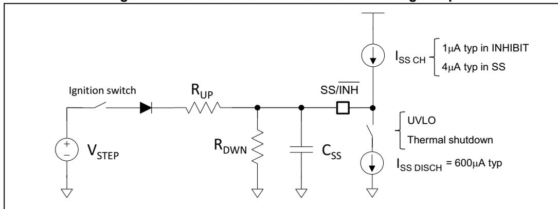
The maximum capacitor value has to be limited to guarantee the device can discharge it in case of thermal shutdown and UVLO events (see [Figure 9](#)), so restart the switching activity ramping the error amplifier reference voltage.
