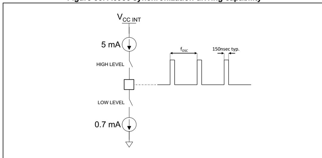
In order to safely guarantee that each regulator recognizes itself in SLAVE mode during the normal operation, the external master must drive the SYNCH pin with a clock signal
