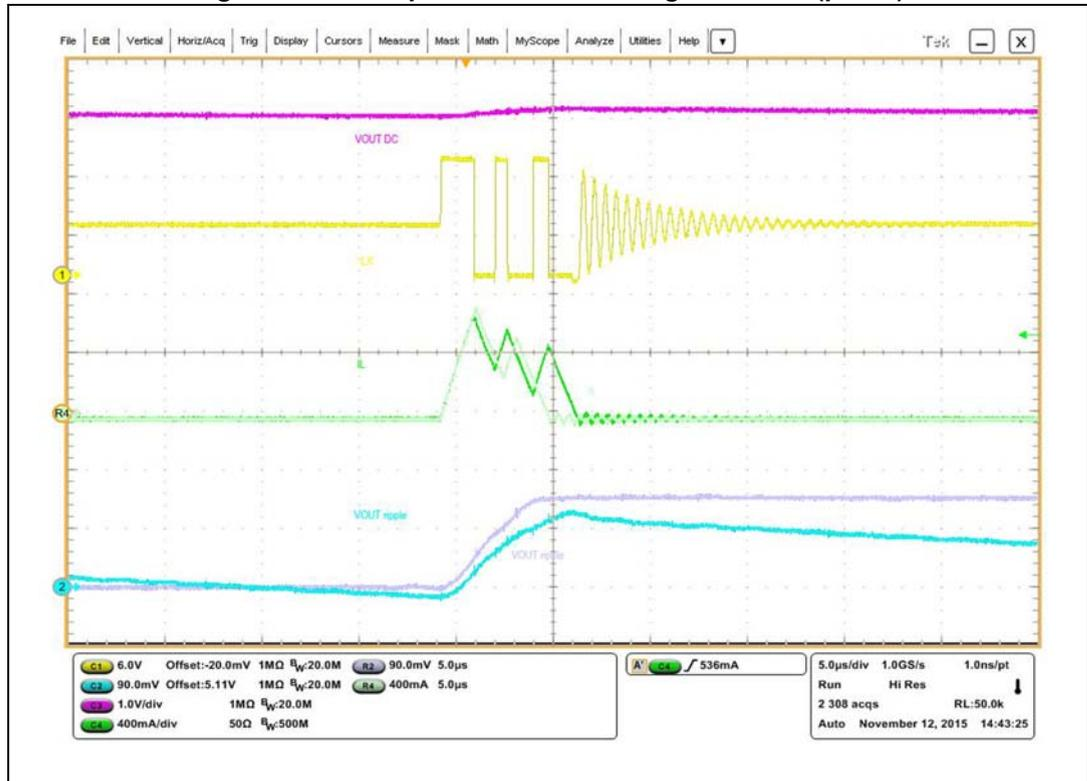
Figure 16. LCM operation over loading condition (part 2)
